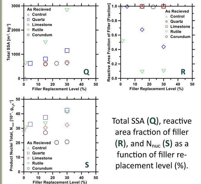
Total SSA (**Q**), reactive area fraction of filler (**R**), and N<sub>nuc</sub> (**S**) as a function of filler replacement level (%).
