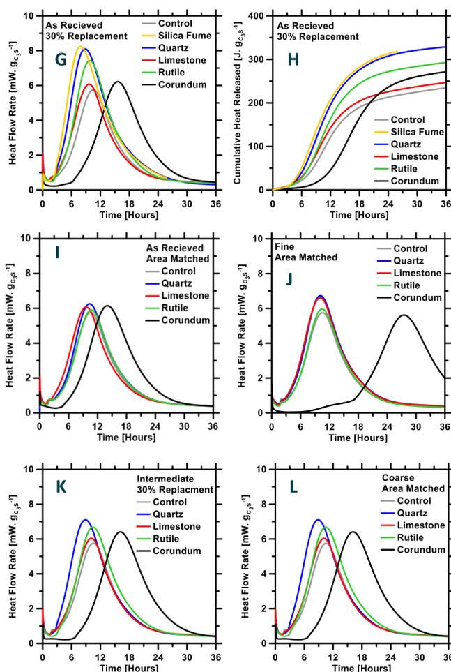
Calorimetry results for as received 30% replacement systems (**G** and **H**), and the four size classes: as received (**I**), fine (**J**; >20μm), intermediate (**K**; 20-25μm), and coarse (**L**; 25-32μm). Areas were matched to specific surface area (SSA) corresponding to limestone for respective size classes.
