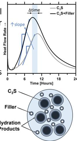
**Study Objective:** to examine the changes in hydration rates as filler type and particle size class is varied.
