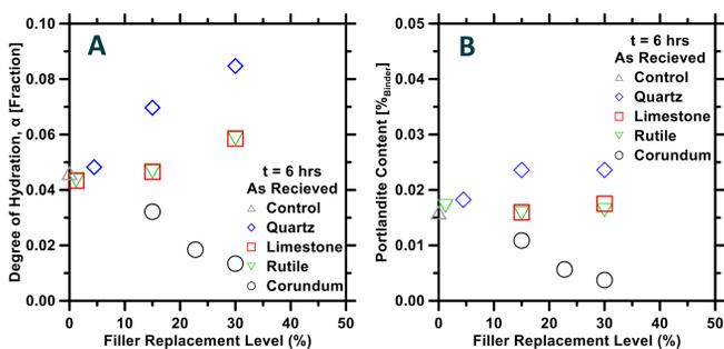
The degree of hydration (DOH) at 6 hours (**A**) and the portlandite content (**B**; %<sub>binder</sub>) determined from SDT and calorimetry experiments.
