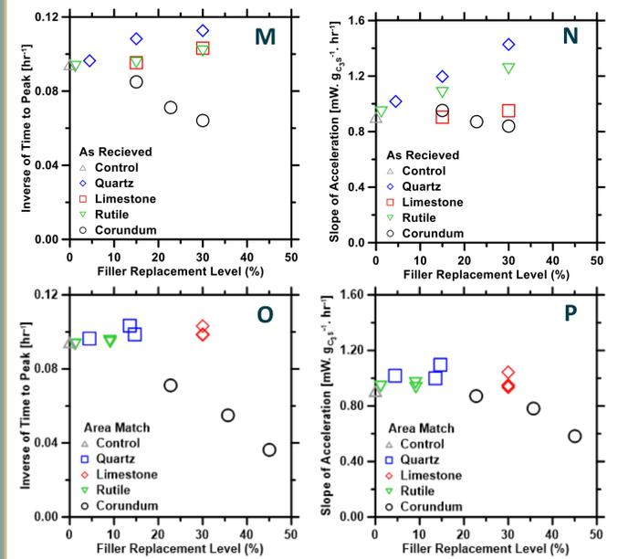
Calorimetry parameters: inverse of time to peak and slope of acceleration as a function of filler replacement level for all as received (**M** and **N**) and all area matched pastes (**O** and **P**), respectively.
