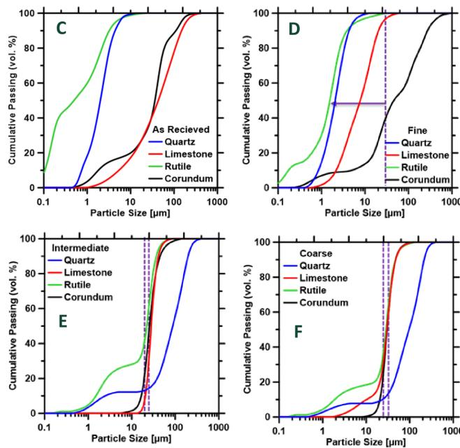
Particle size distributions of as received (**C**), fine (**D**; >20μm), intermediate (**E**; 20-25μm), and coarse (**F**; 25-32μm) size classes. The d<sub>50</sub> of C<sub>3</sub>S was determined to be 7.73 μm.
