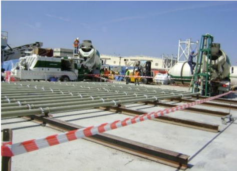
Figure 6. Saudi Readymix pumping simulation setup
