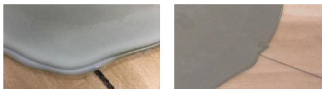
(a) Without CNTs (Mix C15) (b) With CNTs (Mix C13)
