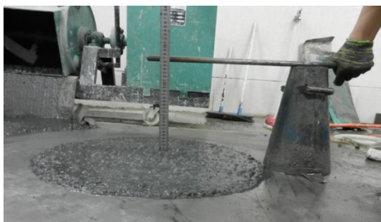
Figure 1. Slump test on Self-compacting concrete
