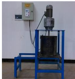
(a) The draft of the abrasion testing machine (b) The abrasion testing machine
