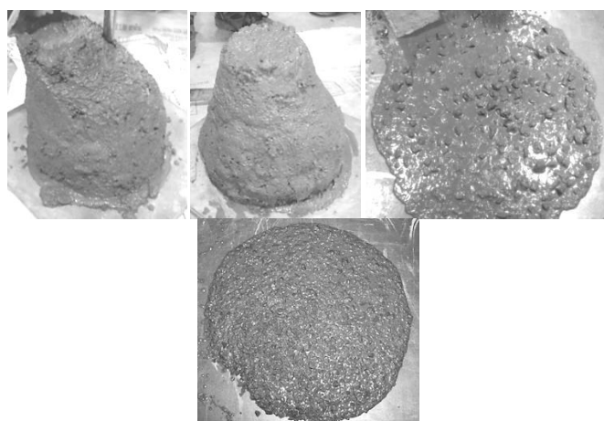
a) NC-Shear slump b) NBC-True slump c) SCC-Slump flow patty d) SCBC-Slump flow patty
