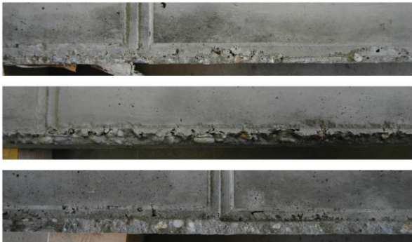
Figure 9. Mixture 2 - Gap of 3 mm – 6 mm – 9 mm (top to bottom)
