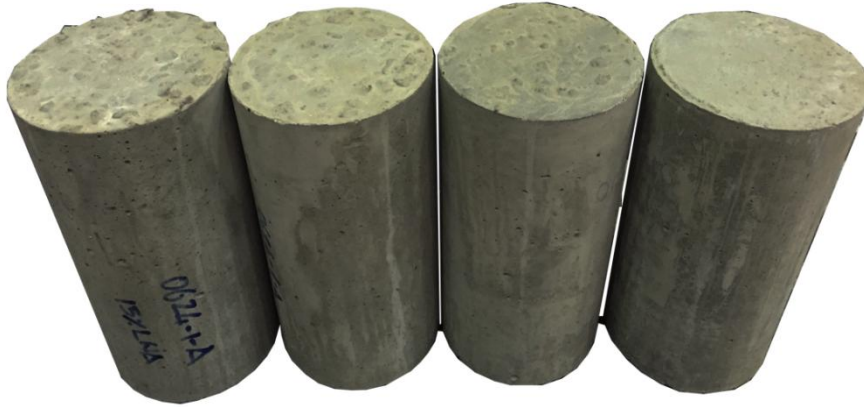
Figure 1: From left to right, concrete cylinders with 15%, 10%, 5% and no-LWA substitution.
