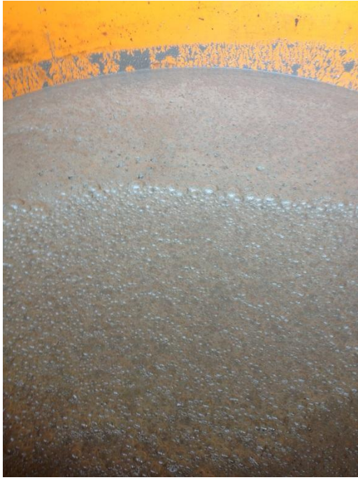
Figure 2: Example of foam formation in batch no. 3 of one truck delivery
