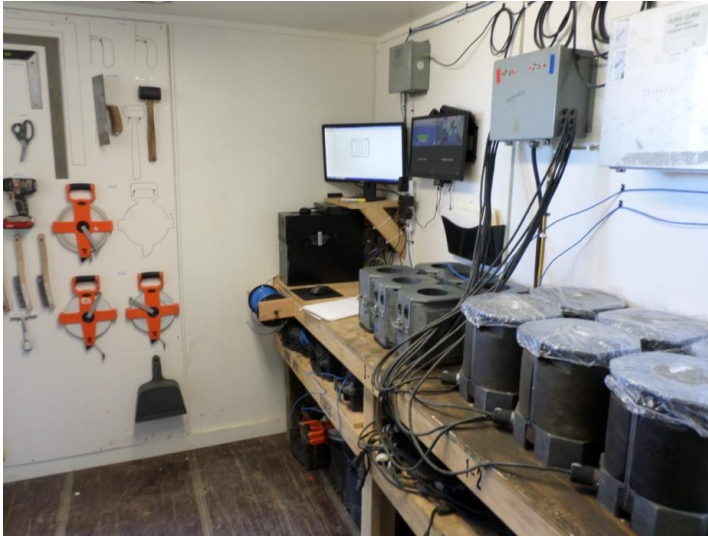
Figure 2. Curing Temperature/Compressive Strength Monitoring System Sure-Cure
