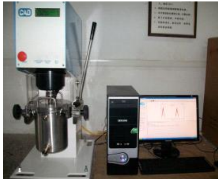
Figure 1. The RCAD400 rheometer used in this study
