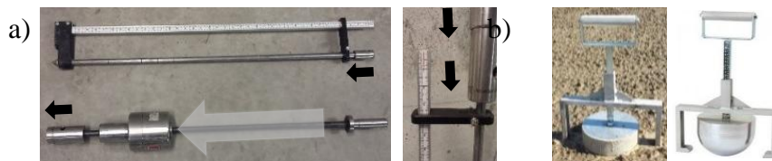
Figure 1. Measurement of the consolidation of CLSM, a) dynamic cone penetrometer, b) ball drop (Kelly ball)
