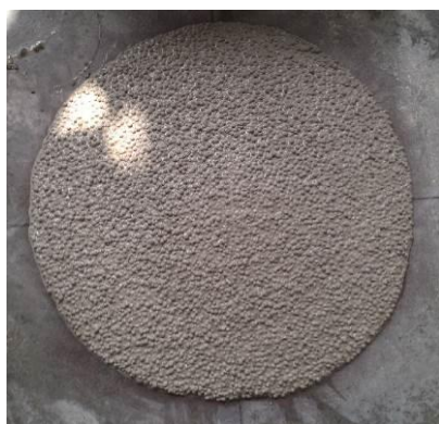
Figure 2. Slump test of M3
