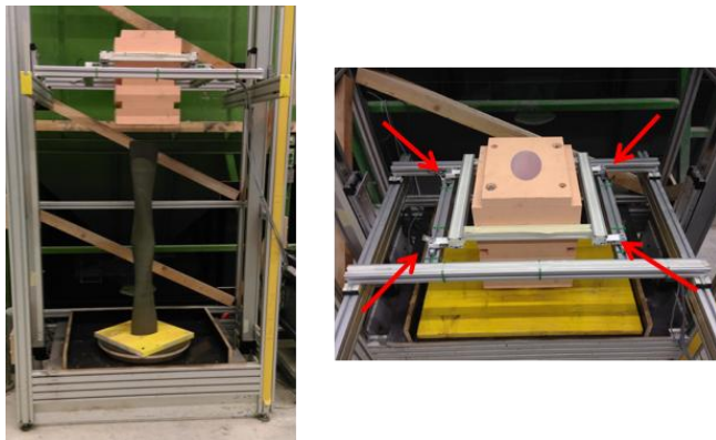
Figure 2. Robotic assembly for Smart Dynamic Casting. Rigid formwork translates vertically, while a rotating table underneath allows rotational deformation. Arrows on picture to the right indicate positions of load cells to measure friction force.
