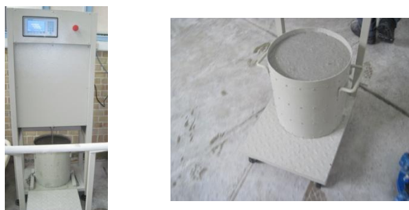
Figure 1. Rheometer for determining the rheology parameters
