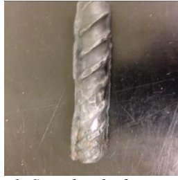
Figure 1. Sample of rebar corrosion
