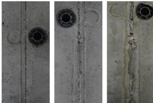
Figure 7. Mixture 3 – Gap of 2 mm – 4 mm – 7 mm (left to right)
