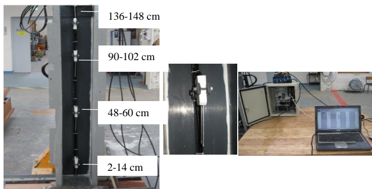
Figure 2. Static stability set-up, conductivity probe, and data acquisition system
