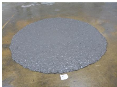
Figure 5. Typical slump flow of developed UHP-GSC
