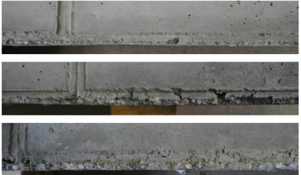
Figure 10. Mixture 3 – Gap of 3 mm – 6 mm – 9 mm (top to bottom)
