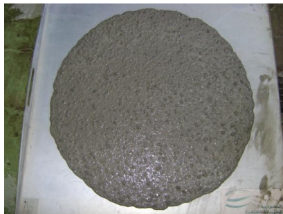
Figure 5. SCC slump flow
