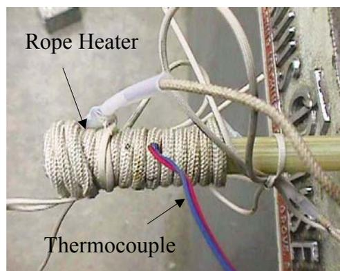
**Fig. 3** - Heating of GFRP bar
