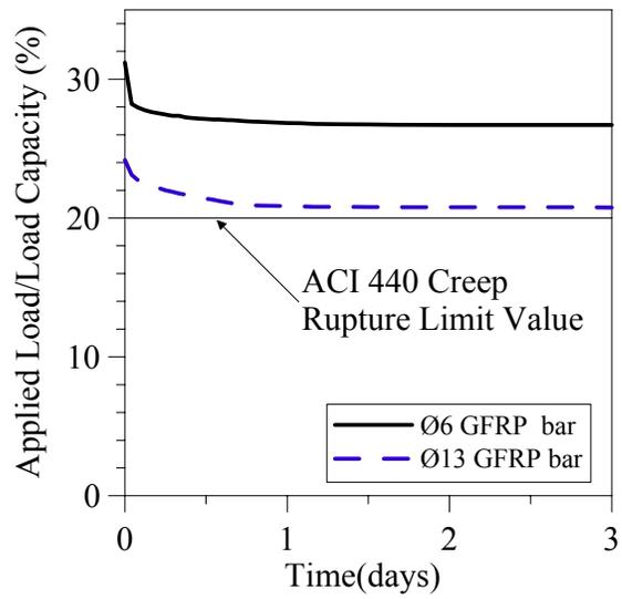
**Fig. 7 - Load relaxation of GFRP bars**
