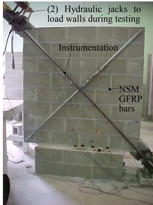
**Fig. 8** - Testing of retrofitted masonry walls with prestressed NSM GFRP bars
