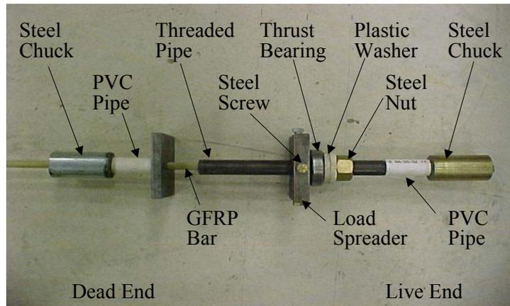
**Fig. 1** - Hand-held device components
