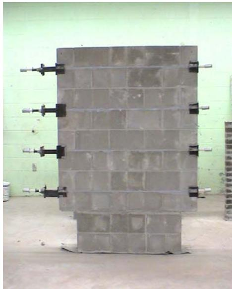
**Fig. 5** - Assembled system in a masonry wall
