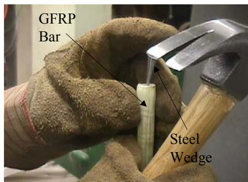
**Fig. 2** - Inserting steel wedge in GFRP bar
