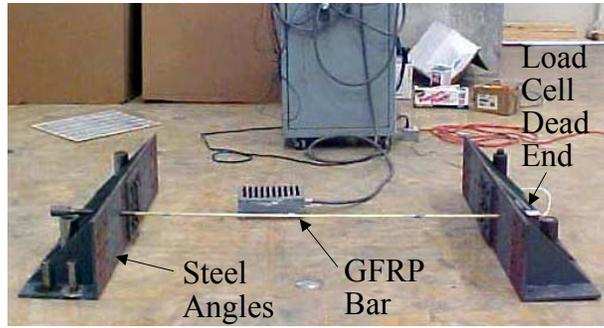
**Fig. 6 - Test setup for component evaluation**
